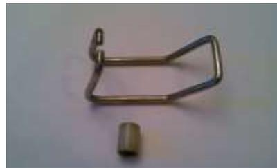
2. Once the handle is removed the only thing preventing the bailer slide from dropping out of the bottom is the 1/8 in. lip at the rear top of the bailer slide. Carefully use vise grips or pliers to bend it straight. If the bailer is down in a hole in the floor the lip maybe difficult to get at.
