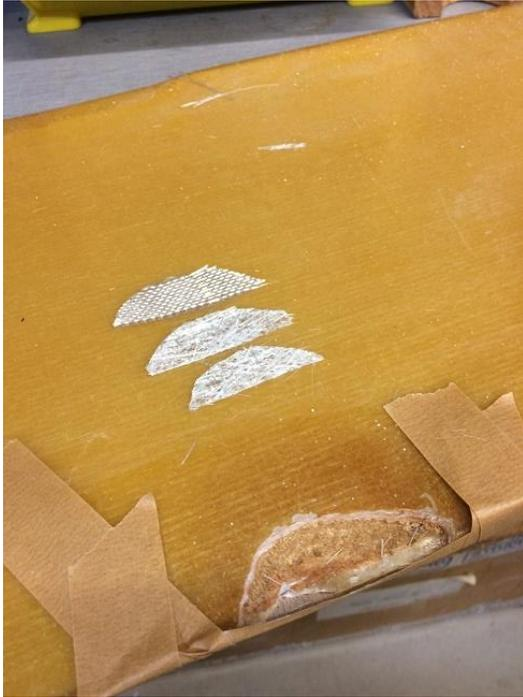
*Damage prepared for repair. Notice the bevel in the repair edges and the uniform shape. The Tape along the underside of the repair will act as a dam to help shape to edge of the repair.*
