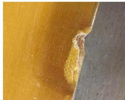
*Damage to be repaired Notice the irregular shape and area where the glass is pulling away from the foam core.*
