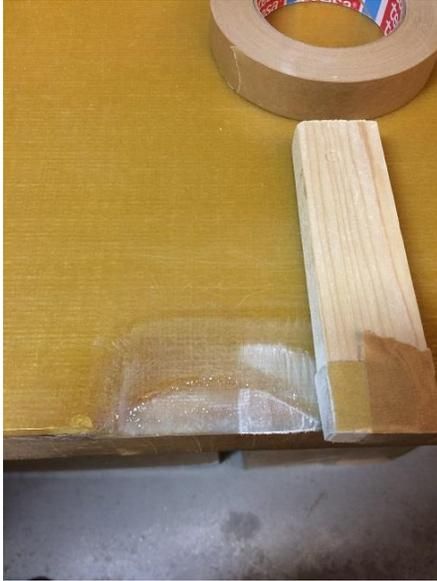
time and wipe the repair often with a damp rag to remove sanding dust. Once the repair is nearly blended with the area use 220-600 to final sand the repair. Use water as a lubricant to keep the sandpaper from clogging.
