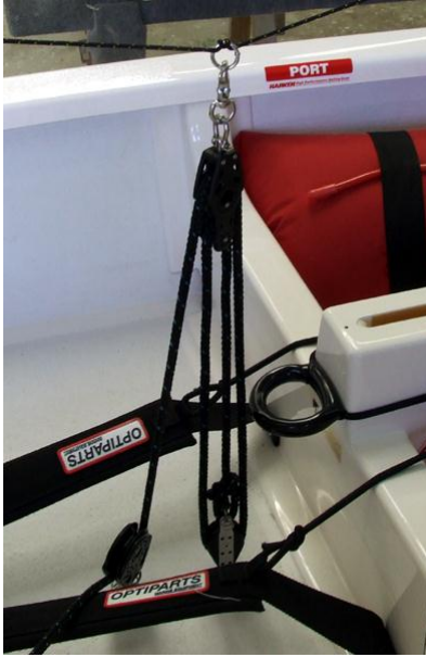
The basic 4:1 system with a Harken 40c fiddle at the boom and a big bullet single with becket mounted on the deck.
