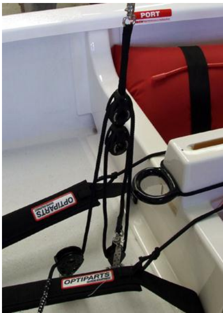
The 4:1 system with a quick release option. MCL01-2 daisy chained 40c blocks at the boom and a big bullet single with becket mounted on the deck.
