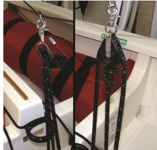
Examples of the wrong and right way to connect the mainsheet to the top block.
