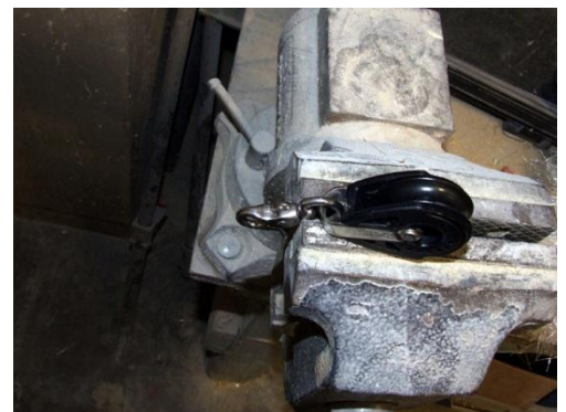
A simple bench vise can be used to lock the swivel
