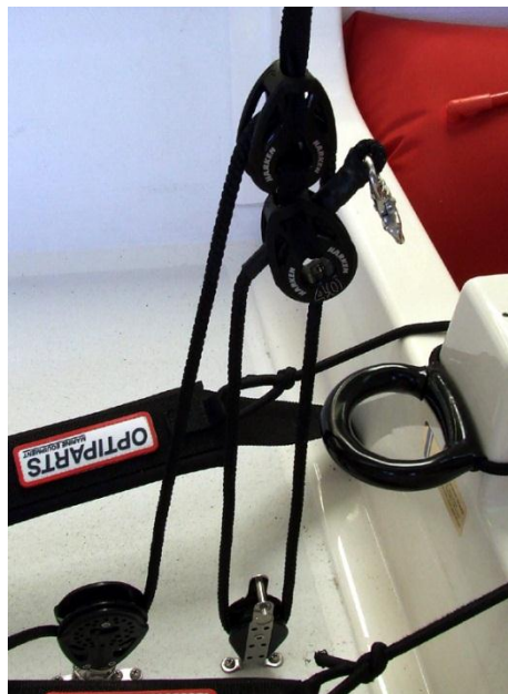
The 4:1 system with a quick release option. MCL01-2 daisy chained 40c blocks at the boom and a big bullet single with becket mounted on the deck.
