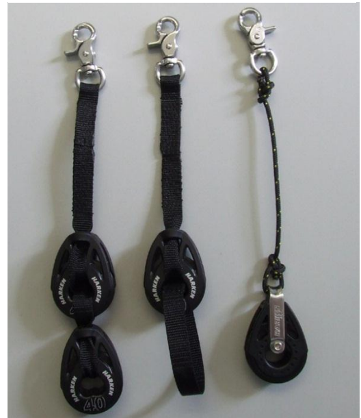
3 examples of boom blocks with strops: MCL01-2 daisy chain for a 4:1 system, MCL01 single block for 3:1 system, homemade version using an EX1372 shackle and EX1308 Harken 40C block.
